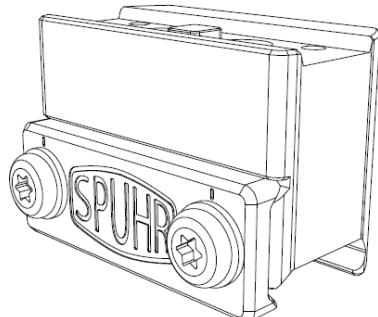
The SM-series of Aimpoint T1/T2 mounts was designed to be the most rugged mount possible. The mount consists of a mount body, a rail clamp, a set of clamping screws with washers, and five M3x6 Tx10 Torx head screws for attaching the Aimpoint to the mount.
