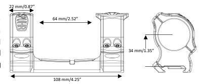
The SCT-3006D Interface Mount features two Spuhr Interface™ Top Covers, which can be installed as to position any of more than 40 different accessories in either the 12 or 3 o'clock position.
